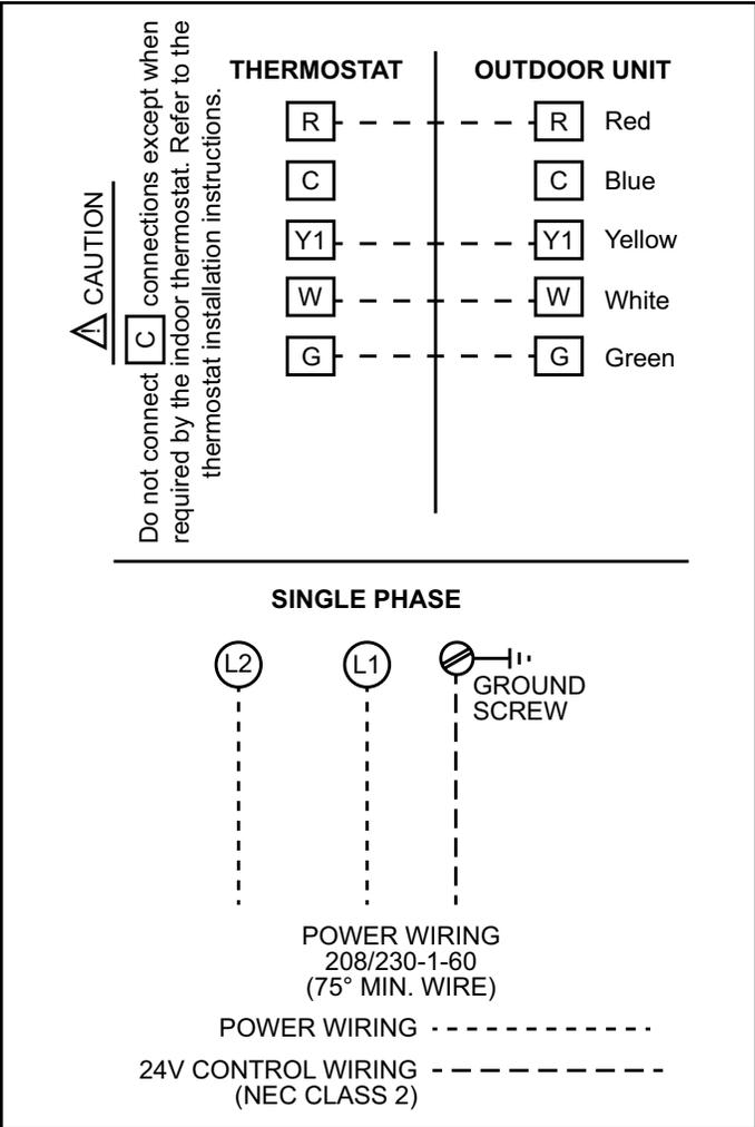
**Figure 5. Typical Wiring Connections**
