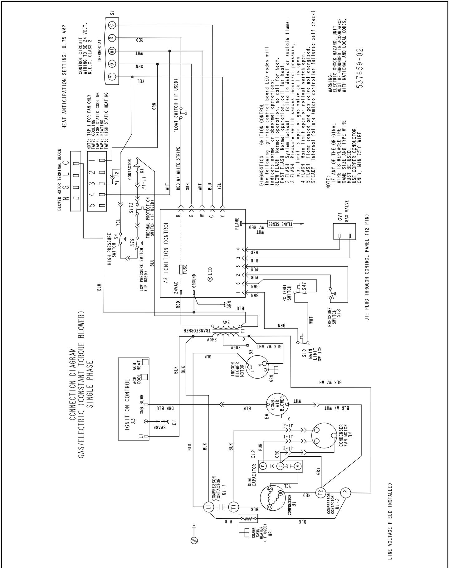
Figure 7. Wiring Diagram – Single Phase CT
